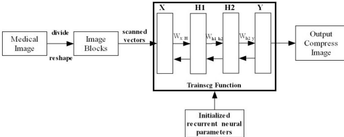
Figure 1. Block diagram of The Compression model
