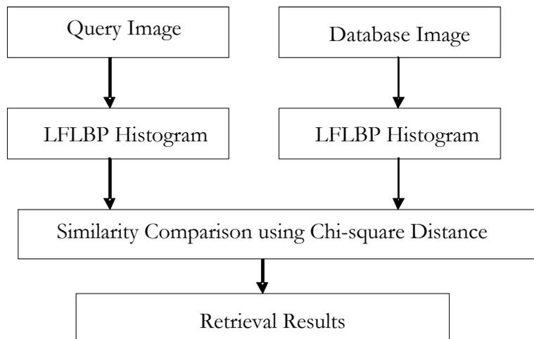
Figure 5. The Proposed CBMIR system using LFLBP Descriptor
