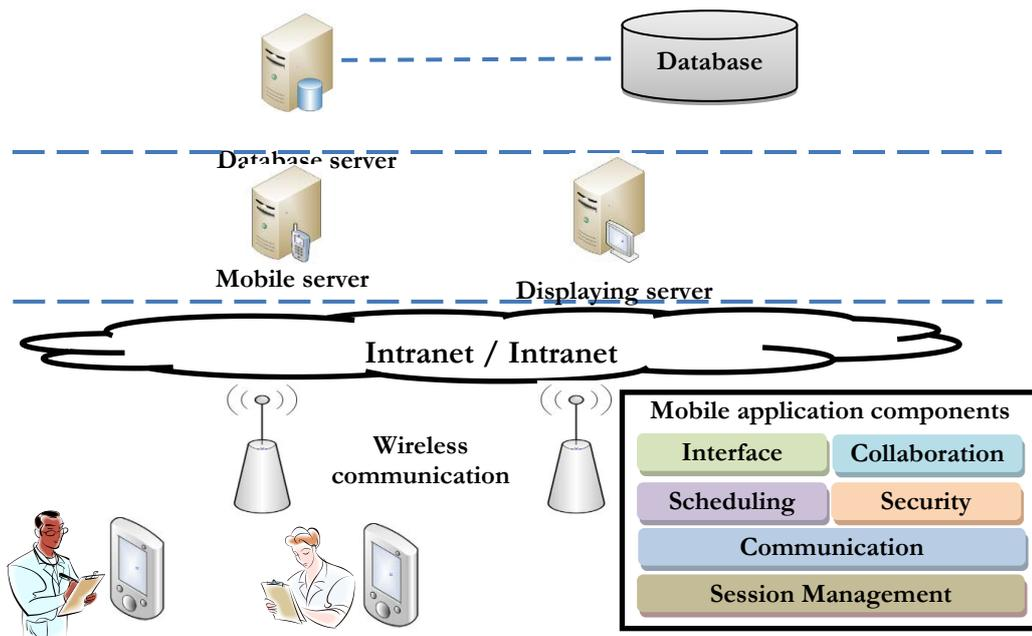
Figure 2. Software architecture
