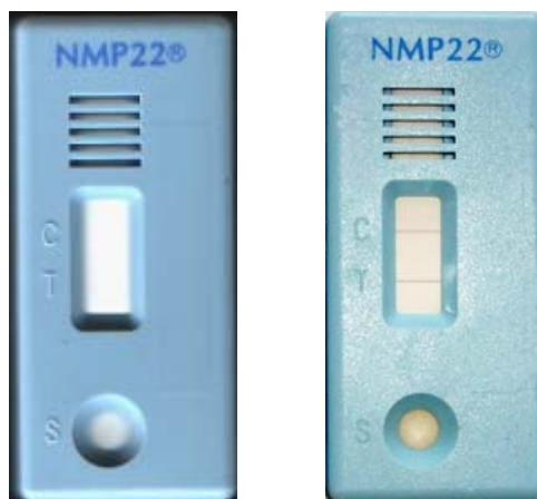
Figure 1. The NMP22 Bladder Check OncoScan test (blank test – left hand picture and positive test – right hand picture)
