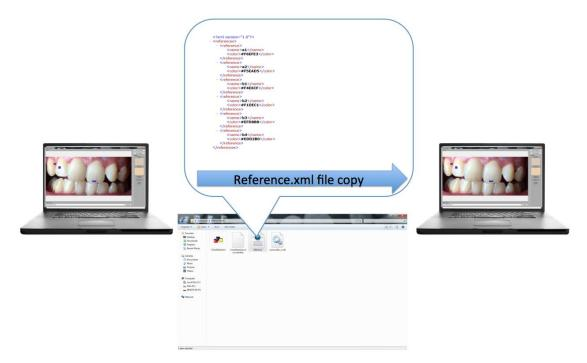
Figure 4. Transfer color keys from a computer system to another
