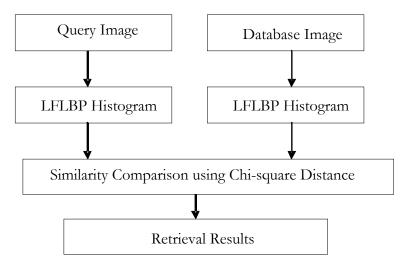
Figure 5. The Proposed CBMIR system using LFLBP Descriptor
