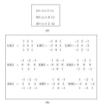
Figure 1. Laws Masks. (a). Basic 1×3 Masks. (b) 3×3 Masks
