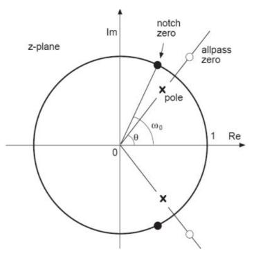
**Figure 4.** Poles and zeros of the notch filter G(z)
