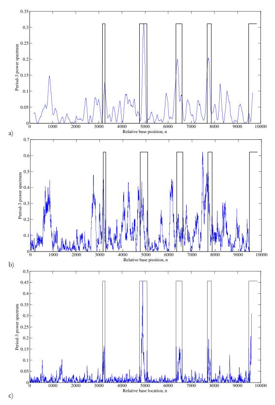
**Figure 5**. The algorithm result for detection of the exon regions on the gene sequence F56F11.4. (a) DFT, (b) MS-filter and (c) Proposed algorithm.
